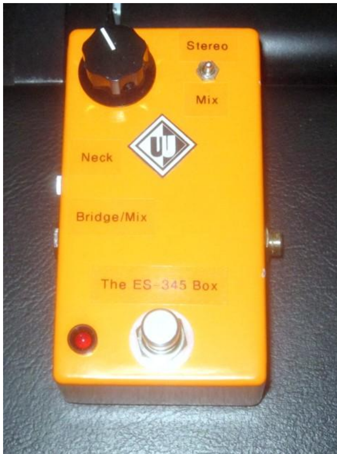
Figure 22 – My home brew stereo guitar interface pedal
