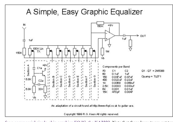
Here is a circuit diagram of a simple to build graphic EO. Notice that the circuit is very repetitious. the frequency selective elements are made of capacitors and "gyrators" that simulate the response of grounded inductors. These make the circuit free of real inductors, and are simpler to tune if tuning is needed. With standard value components, the frequency ranges come out a bit imperfect, but this is usually not noticeable in real situations.
