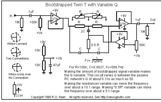
We can simply put a volume pot on the output of opamp U1b, leaving it just functioning as a buffer to keep the T unloaded, and use another opamp to drive the bootstrapping point of the T. This opamp is driven from the wiper of the pot, however. You can see that if the pot is fully up, the T is getting full bootstrapping for a Q of 50 or so, and when the pot is full down, the output of the second opamp is
