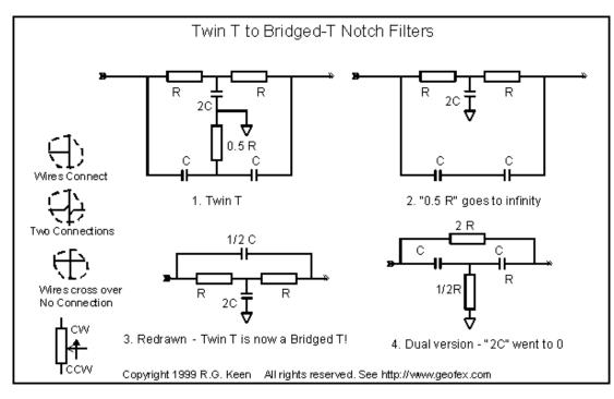
You've probably seen other RC filters used for scoops and notches. There are several of these, but one that comes up pretty often is the Bridged-T. This is a very close relative to the Twin T, as you can see from the sketch. If vou take a basic Twin T and let the 0.5R leg resistance go to infinite resistance, and then combine the two series capacitors into one cap of 1/2 C, you get the Bridged-T. This thing is amenable
