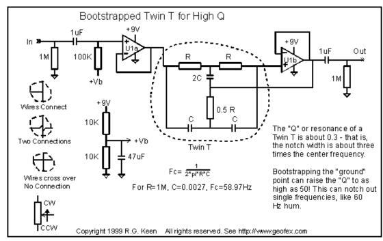
The section shown in the dotted line is a basic Twin T, if you ignore the opamps and connect the center junction of the 2C/0.5R leg to ground. The twin T is one of the very few filters made from only resistors and capacitors that can cause an infinitely deep notch or attenuation. That is, at the exact center of the frequency dip it causes total attenuation of the signal.
