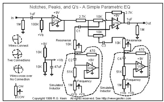
inductor shown, the inductance is equal to the value of C2 times the 470 ohm resistor times the series resistance of the 51K and the setting of the 1M pot. Or more prosaicly, Leff = R1\*R2\*C, where R1=470, R2= series resistance, and C= C2's value.
